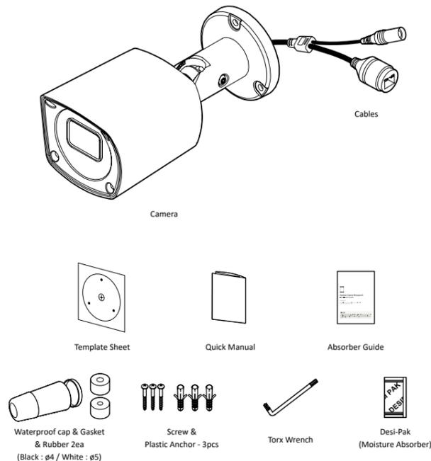
Note : Cable thickness 4.5φ to 5.5φ uses a black rubber, and over 5.5φ uses a white rubber.
